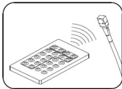
infrared sensor for RGB lights must not be hidden as otherwise remote control will not respond
